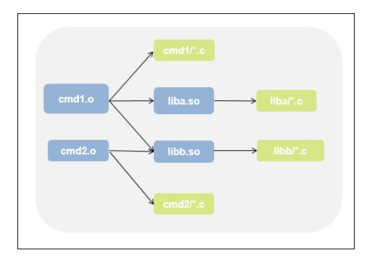
Build your source code by using the makefile. Use the -B flag to ensure full build.
